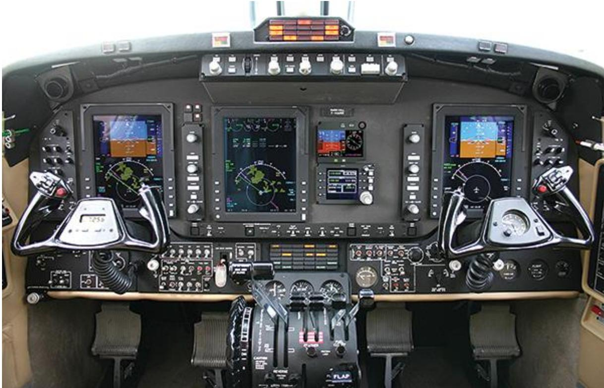
*On Saturday, Dec. 11, 2021, I had the pleasure of trying out the ThrustSense Autothrottle system for the first time. IS&S is the abbreviation for Innovative Solutions and Support, the company that designed, tested and certified this system that adjusts power lever position to maintain a torque value or an airspeed value that the pilot desires.*
