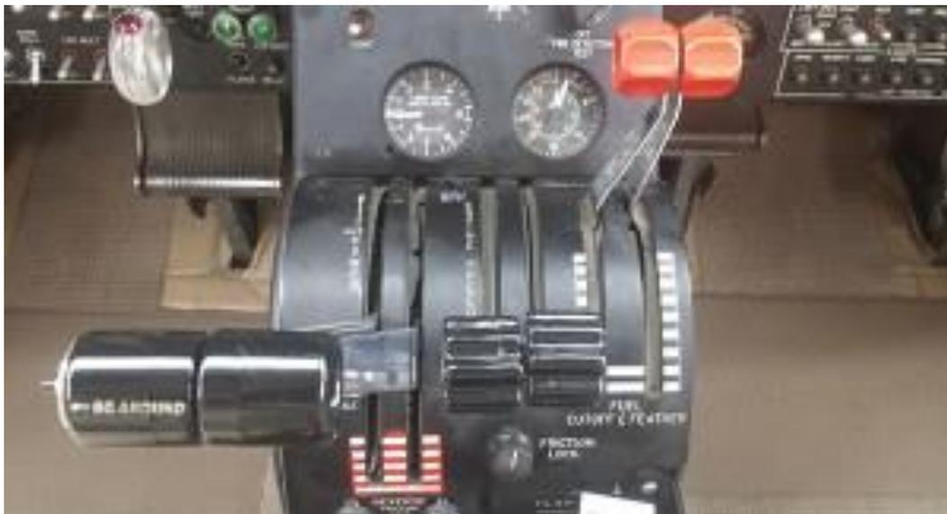
*The power quadrant levers in the B100 changed to being called Power, Speed and Fuel Cutoff & Feather*
