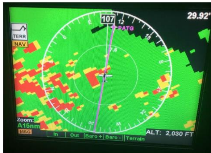
Figure 9. Photograph of the simulator's Garmin MX 20, using the terrain function.
