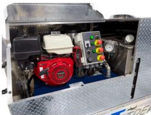
12 HP Honda Engine & Control Panel
