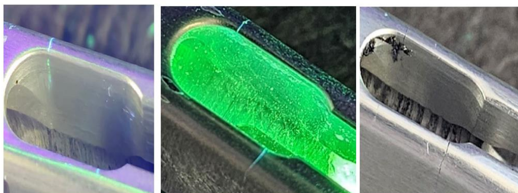
Figure 2. Sample cracks found with visual and fluorescent penetrant inspection.
