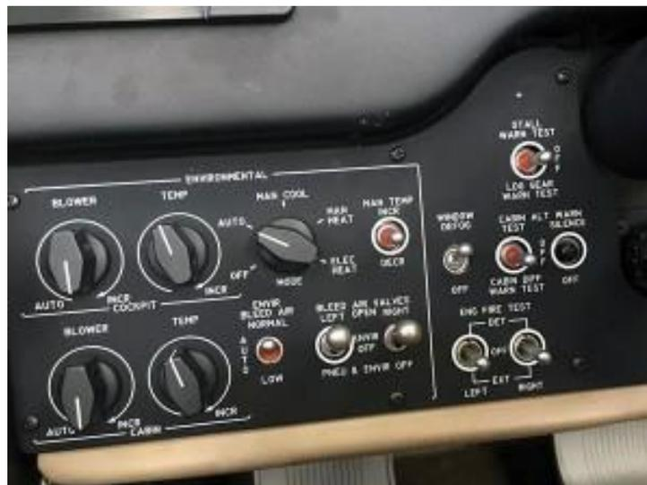
*Notice that in both models the pilot has manual control of Bleed Air temperature but not “Auto,” without generators. We will receive inflow for pressurization and heating only from the left side’s Flow Pack. A confusing realization in the C90A system is that both the Air Conditioning and the Electric Heater systems receive power from the Center Bus ... and it is not a bus that is shed! Rest easy, however – a special circuit causes those two heavy-load items also to be unavailable.*
