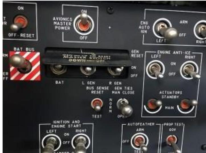
*Keep in mind that the non-circled components, the items that are shed, can be easily brought back to life by the simple action of moving the "Gen Ties" switch up to "Man Close." (It then springs back to Norm while giving you an advisory annunciator of "Man Ties Close").*
