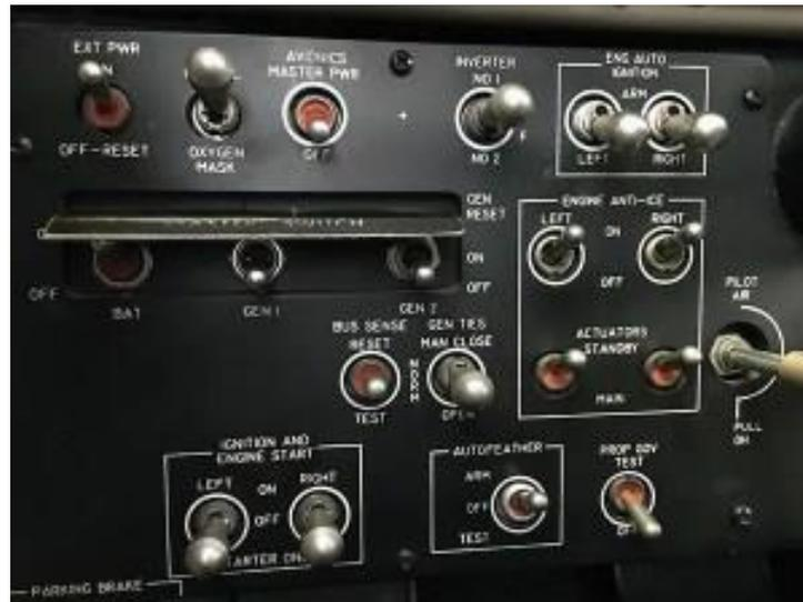
*Notice the ones on the “Engine Anti-Ice” switches. Get your black Sharpie felt-tip pen out and mark over them ... they should not be there! Notice that there are no circles around the “Actuators” switches. Well, if neither Standby nor Main motors are powered following load shedding, then how can Engine Anti-Ice function? It cannot, so the white circles are a design flaw / manufacturing mistake.*
